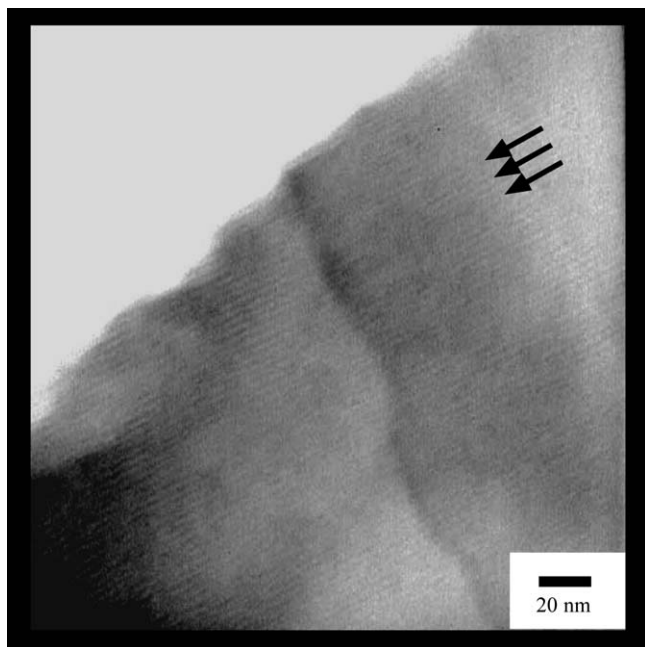
Fig. 6. A transmission electron micrograph of the titania/mesoporous silica composite film prepared by optimal condition. The amount of \text{TiO}_2 : 5.0 wt.%. Spincoating rate: 5000 rpm. Drying temperature: 160^\circ\text{C} .
